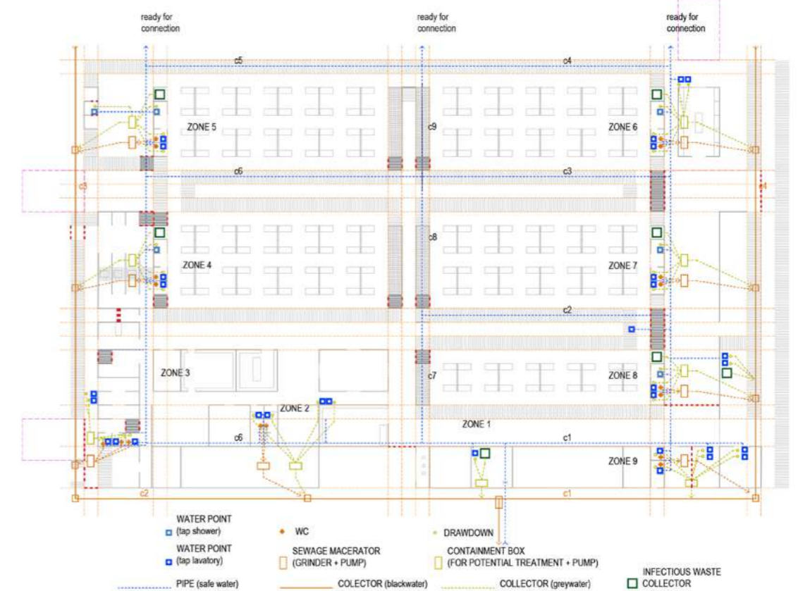
Fig. 8.6 Proposed sanitation system for Model M (100 m × 80 m) 160 moderately ill inpatients + 20 specific inpatient profile area beds + 60 staff
