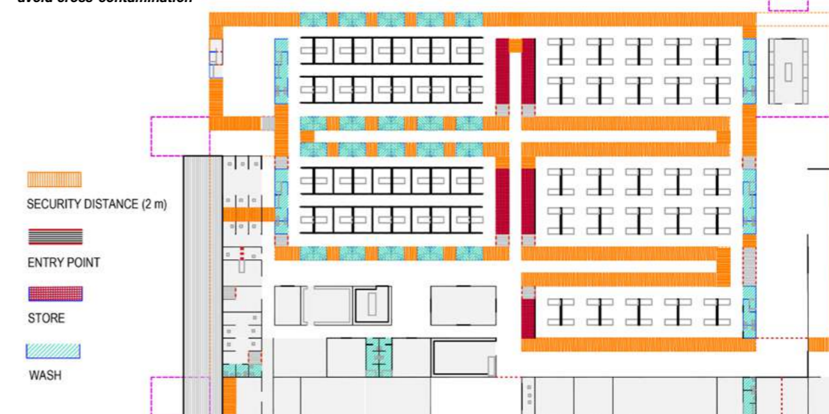
Fig. 6.3 Suspected cases' ward (left) and confirmed cases' ward (right) in the proposed set-up. Note that in the left ward, there are only 20 beds in separate cubicles, to ensure individual isolation and avoid cross-contamination
